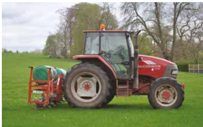
Soil aerator. Image © Eden Rivers Trust
