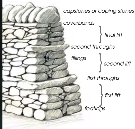
Features of a dry stone wall
