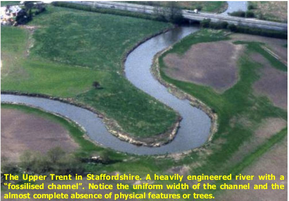
**The Upper Trent in Staffordshire. A heavily engineered river with a "fossilised channel". Notice the uniform width of the channel and the almost complete absence of physical features or trees.**
